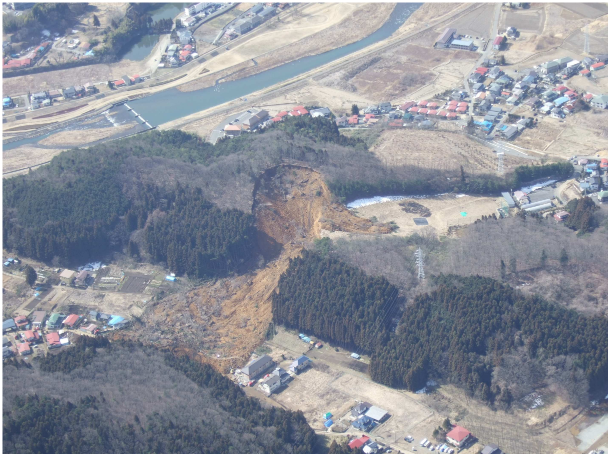
Figure 1. A typical catastrophic landslide induced by an earthquake on a slope of pyroclastic fall deposits. The Hanokidaira landslide induced by the 2011 Tohoku earthquake. (Photo courtesy: National Institute for Land and Infrastructure Management and Public Works Research Institute).
